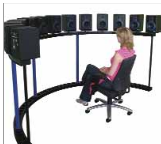
180 degree speaker array for assessing hearing directionality. Only available to special order.
