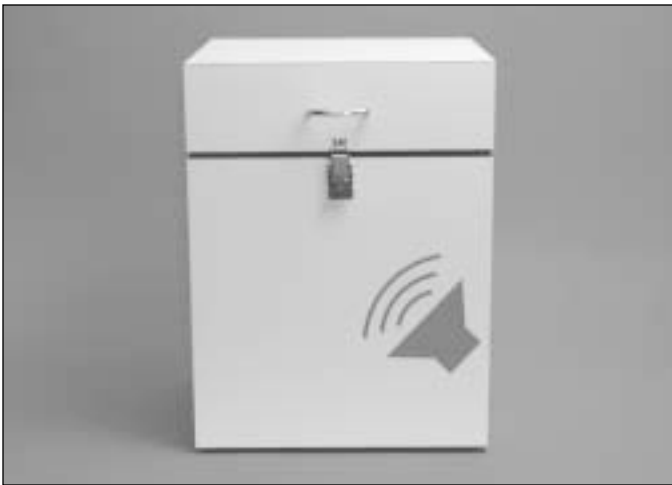
Figure 1—Sound chamber with speaker mount
