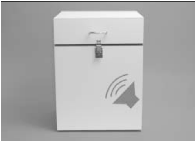
Figure 1—Sound chamber with speaker mount
