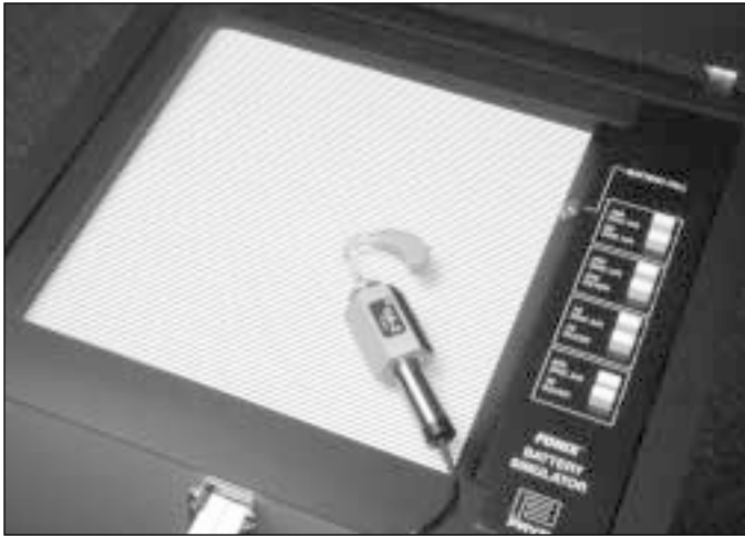
Figure 3A—Reverse measurement in 6050 sound chamber
