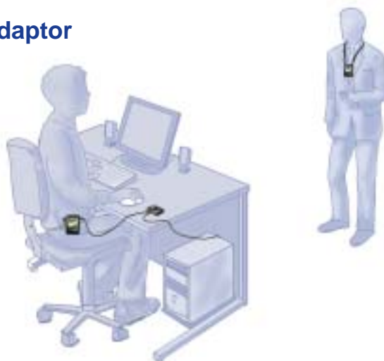
Group use with the computer connected to the environmental microphone input of the radio aid receiver and the transmitter worn by the tutor as usual. The receiver 'Tx' vol control adjusts the tutor volume and the 'E' volume control adjusts the computer volume.
