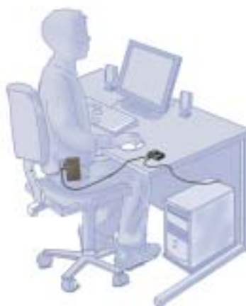
Group use with the computer connected to the environmental microphone input of the radio aid receiver and the transmitter worn by the tutor as usual. The receiver 'Tx' vol control adjusts the tutor volume and the 'E' volume control adjusts the computer volume.
