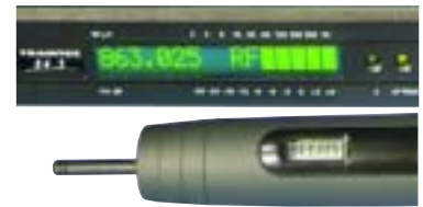
Set of handheld microphone and radio microphone receiver showing matching frequency
